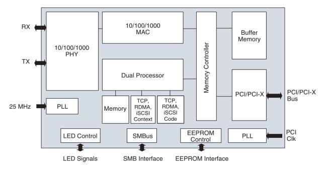
The **BCM5706** provides a fully integrated Layer 4 and Layer 5 solution - TCP/IP, RDMA and iSCSI 1.0/iSER along with a complete 10/100/ 1000BASE-T Gigabit Ethernet, IEEE 802.3 compliant Media Access Control (MAC) and Physical Layer Transceiver solution for high performance network applications. By itself the **BCM5706** provides a complete single-chip Gigabit Ethernet NIC with a TCP/IP Offload Engine, RDMA NIC (RNIC), iSCSI 1.0/iSER HBA or LOM solution.
